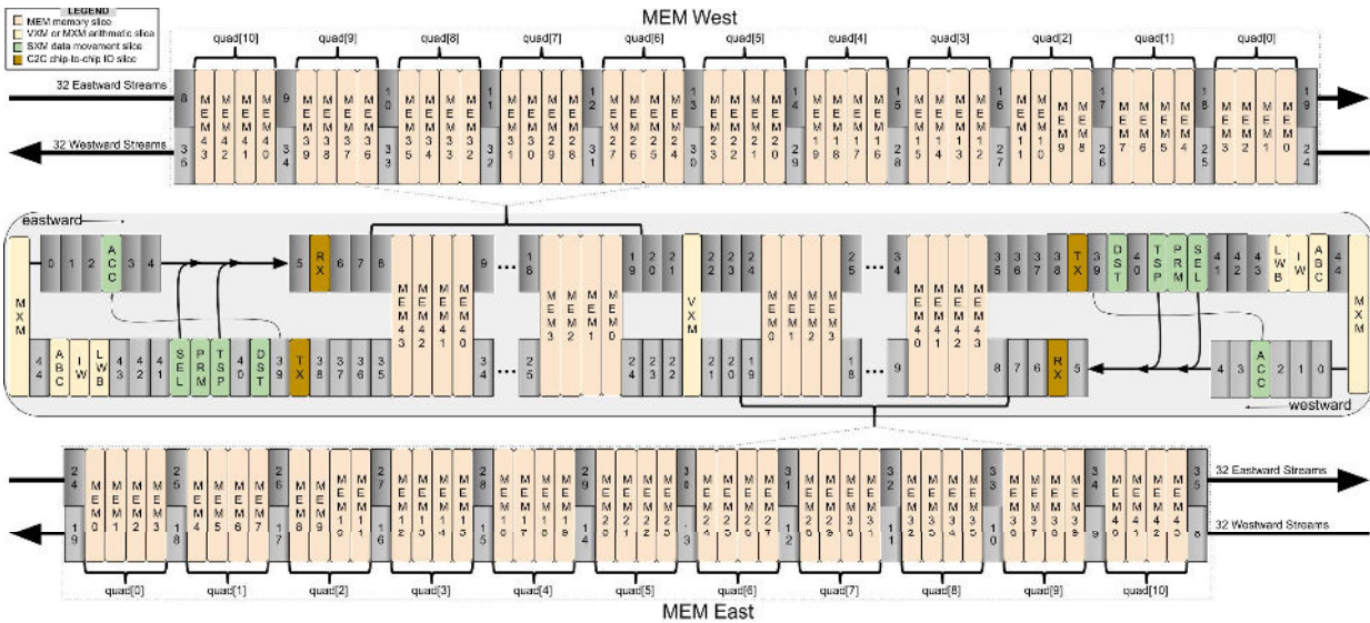
Fig. 4. Stream registers are numbered to show their locations between the functional slices within a superlane.
